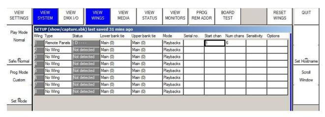
A "D" in the Status Window shows that the panel is detected. It will then control four Playbacks on that Wing. Playbacks can be programmed on MagicQ from the Playback Window.
