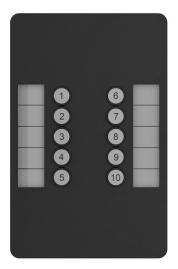
The front panel interface contains 10 10Scene buttons, these have dual colour LEDs used to indicate when a Scene has been stored to a button and when a Scene is active.
