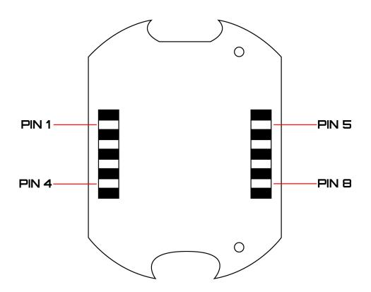
When looking at the rear of the 10Scene Pin 1 is at the top left and Pin 5 at the top right.
