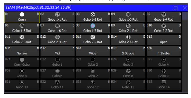
For indexed attributes such as colour wheels and gobo wheels, the button associated with each encoder can be used to bump the attribute value to the next range. Pressing SHIFT and the button bumps back to the previous range.
