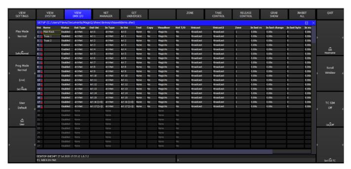
To enable output of channel data select the DMX IO VIEW in the Setup Window. This window enables modification of the inputs and outputs for all the universes. MagicQ consoles support DMX directly from the console or via an external Ethernet to DMX convertor. On MagicQ PC or Mac you can output via USB to DMX interfaces (such as MagicDMX) or via DMX outputs from the Wings.
