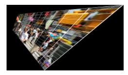
The 8 keystone parameters move the corners of the image within the output screen:
