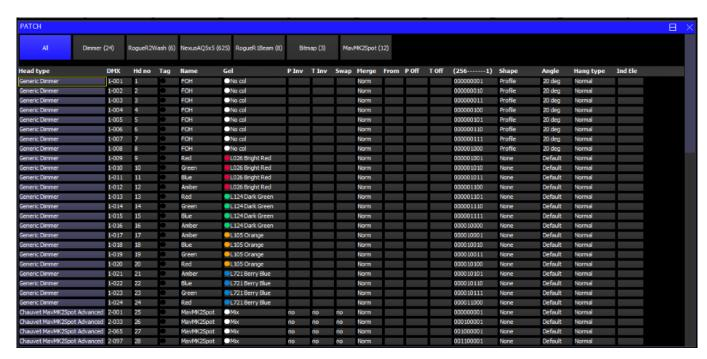
Choose the head you wish to patch by pressing the CHOOSE HEAD soft button. The Window will change to give you a list of heads. Select a head by pressing the touch screen. Alternatively scroll around the Window using the cursor keys, and press ENTER when the cursor is over the correct head.
