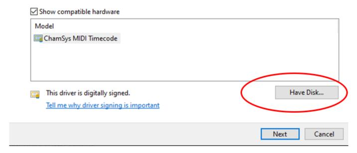
For PC Wing Compacts the drivers are in C:\Program Files (x86)\ChamSys Ltd\Magicq\MagicQ Wing Drivers\PWing Compact\CDM 2.08.24 WHQL Certified\ftdibus.inf
