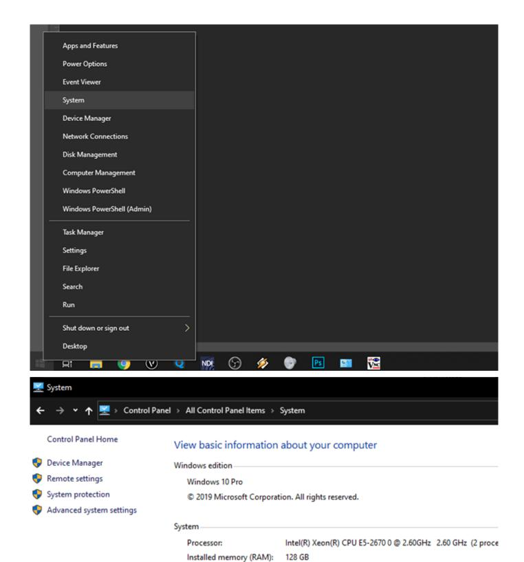
Device Manager lists all the devices on your system. The MagicQ device is normally listed at the bottom under Universal Serial Bus Controllers but it may be under any other section. It may be listed as a ChamSys or MagicQ device or just as a FTDI device. If you can not find it then try disconnecting and reconnecting the USB cable to the device - the listing should update and indicate to you which device is being plugged/unplugged.
