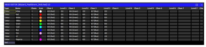
For each Palettes you specify the type (press Enter to swap between the types), the name and the number of channels that make up the Palette. Then for each channel you specify the channel number and the level for that channel.
