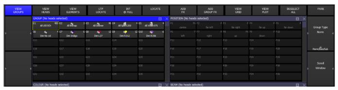
Within the Output Plan window the heads for the previously selected group can be arranged to use with Simple Pixel Map FX. Group grids can only contain heads that are within the Group.
