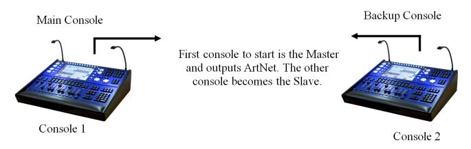
In "Equal mode" all consoles on the network are set to "Hot take-over". At any one time, one of the consoles will run as the master, with all universes enabled. If that console fails, one of the others will take over. It is recommended that you set the "Hot take-over detect time" to different values on each of the consoles to avoid conflict conditions.
