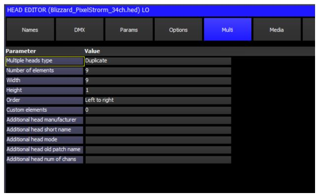
Heads that consist of a single general element in addition to a repeated element are also supported. In these cases two different heads are required – one for the general element and one for the repeated element. The head for the general element is used for patching, and it references the repeated element to enable it to be patched automatically. It is possible to set the Multiple Heads Type field to specify whether the repeated elements are patched before or after the general element.
