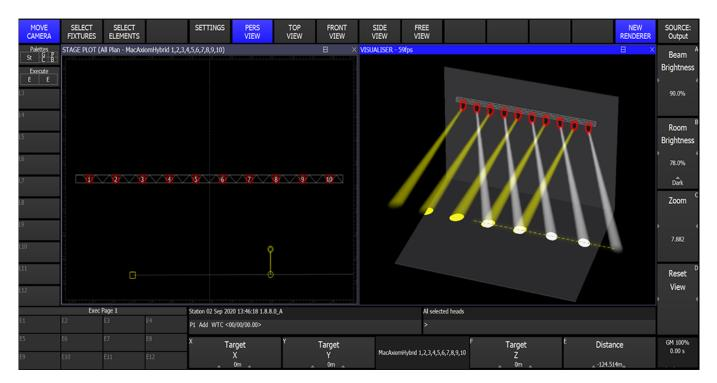
The *Base Position* is the starting position for the heads before they are panned around to focus on the point. If the head has to pan more than 90° from the base position then it will *flip* the head over. The default base position is directly downstage. If the lights flip while they are moving between positions then a different base position may be required.
