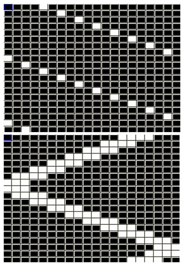
Vert random, Horiz random – enable random movement of elements across the grid. Modify the mode to change thickness of the elements and offset to change the frequency. With this FX it is possible to generate snow and rain type FX.
