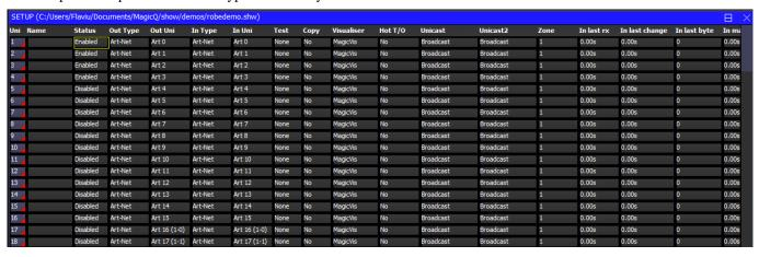
When you set a universe to "Hot Takeover" you must ensure that Input is enabled on that Universe and that it is set to the correct type and universe number – generally the Input should be set up the same as the Output.
