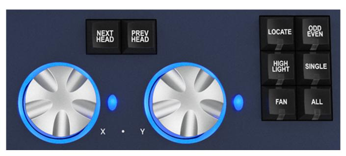
The NEXT HEAD and PREV HEAD buttons are used to select an individual head to modify.
