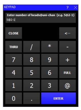
For example to patch 12 Chauvet Professional Maverick MK3 Spots in advanced (39 channels) mode, at universe 1 start address 1:
