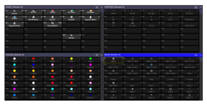
The highlighted window enables controls the soft buttons and rotary encoders. In each of the Windows the X and Y encoders control the most important attributes – Pan and Tilt in Position Window, Col Wheel 1 and Col Wheel 2 in the Colour Window and Gobo Wheel 1 and Gobo Wheel 2 in the Beam Window. In the Beam Window there are more than eight attributes to be controlled – these are accessed using multiple pages of encoders – by pressing the NEXT PAGE soft button.
