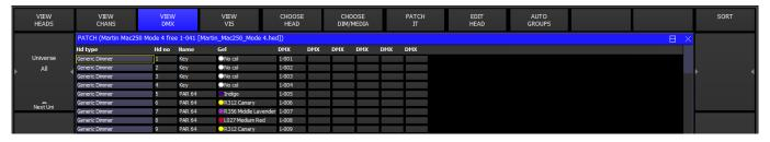
To use this support, patch a Generic Scroller With Dim. This will appear in the View Heads with the DMX address marked as "virtual" and any DMX address you specified when you patched it will be ignored. Change to the View DMX view and specify in the appropriate DMX columns the DMX address of the dimmer and the scroller.
