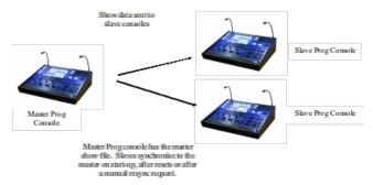
Multi programming enables multiple consoles to access one show file held on the master console with all consoles being able to make changes to that show file. MagicQ ensures that the slave consoles are synchronised to the master console show data. Updates from any console are synchronised across the network.
