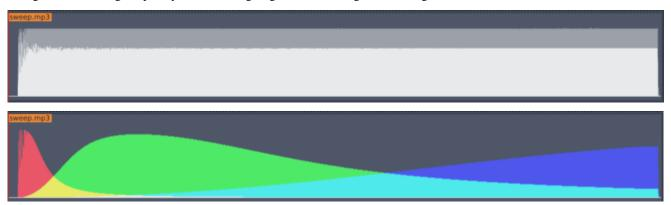
The Cue Stack audio file will always start at the 00/00/00.00 timecode value as this is started when the Cue Stack is activated. Cue Audio files will move in conjunction with their corresponding Cue in the above row.
