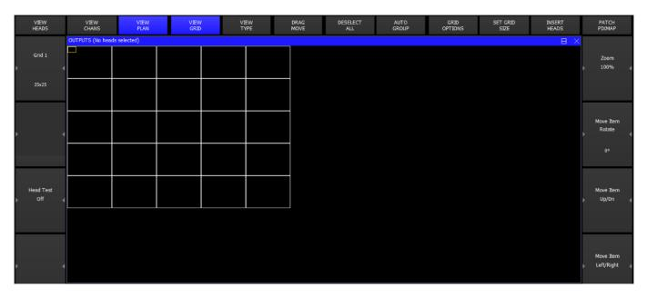
Note that it is not necessary to allocate a head number to every position in the grid – so if your LED heads are placed at weird angles you can make a grid with the LED placed as you would see it. Multiple grids can contain the same head numbers – so it is possible to have one grid with the LED tightly packed and anther representing how they are really spaced out.
