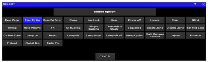
There are special functions for controlling universe zones – enabling, disabling and setting the hot takeover state. These enable complete control of complex DMX routing from a simple interface.
