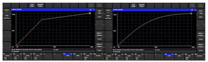
To name a curve first type type the required name then press Set, then encoder A.
