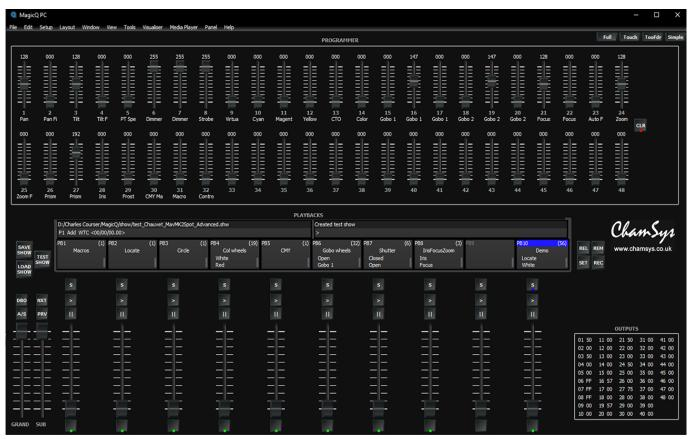
The Playback faders are automatically set up with some useful functions including Macros for Lamp On, Reset and Lamp Off, Locate and Movement, Colour, Gobo and Strobe tests.
