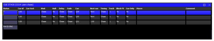
The timing mode can be changed, so that the Cues play back in a theatre style using the GO / STOP buttons. Select the VIEW OPTIONS view and press the CUE TIMING and CHASE TIMING soft buttons to modify the timing mode.
