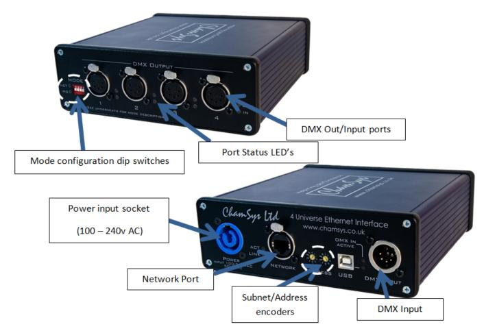
For simple Art-Net or ACN to DMX output conversion on the SnakeSys B4 the DIP switches/rotatory encoders can be used to quickly configure the device for this mode.
